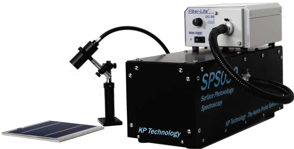
Surface Photovoltage Spectroscopy SPS030 pictured with silicon solar cell sample
