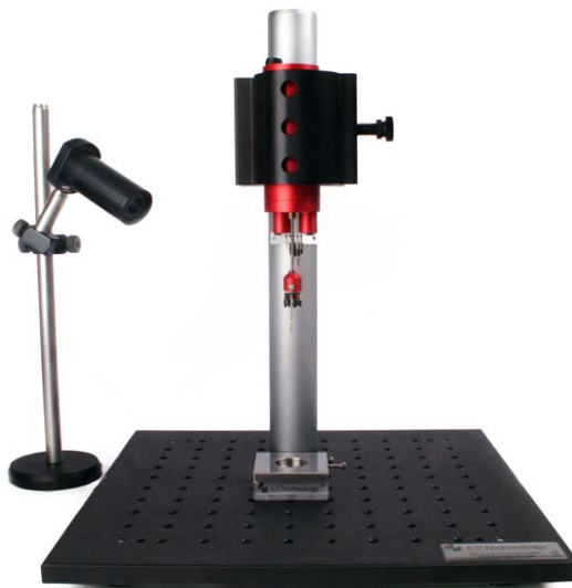
Figure 1. KP Technology KP020 with SPV010
